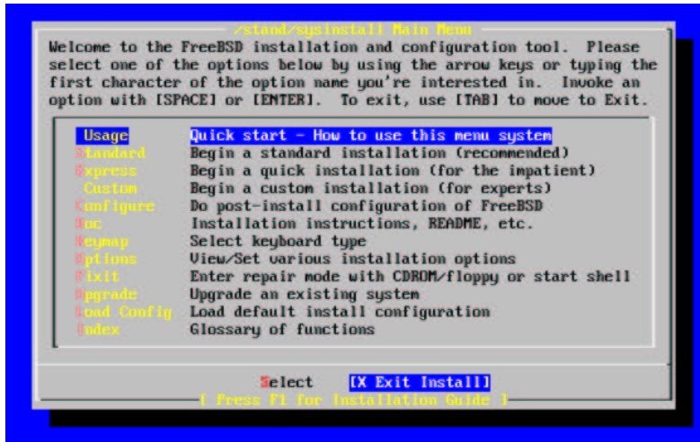
Figure 2-7. Select Sysinstall Exit
